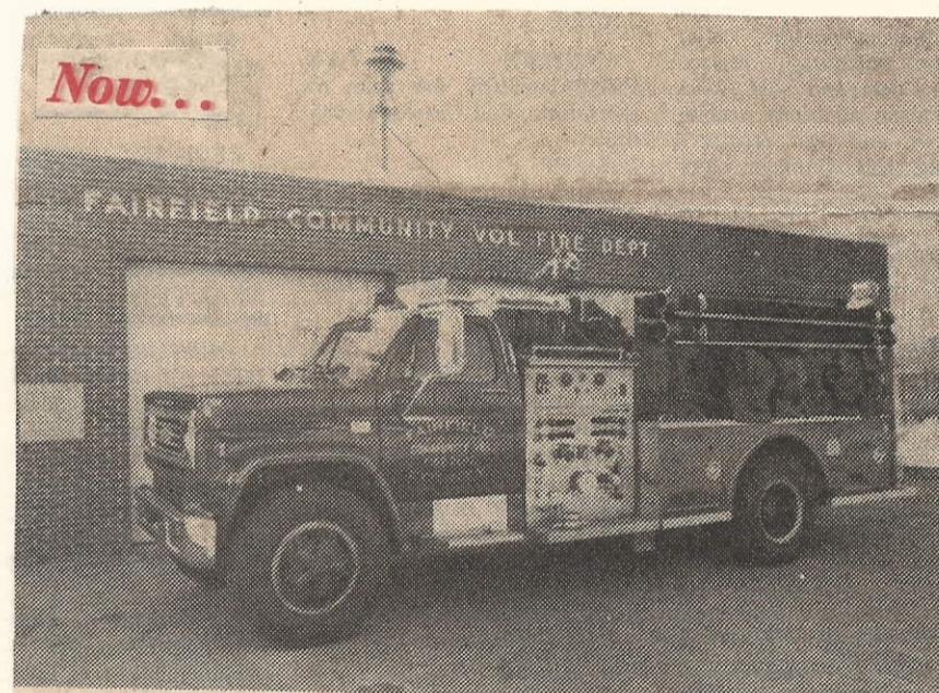
These days, the pride of Community's fleet is this 1984 Chevrolet, which has a 1,000 gal. per minute pumper, and meets all state and federal specifications for firefighting equipment.
