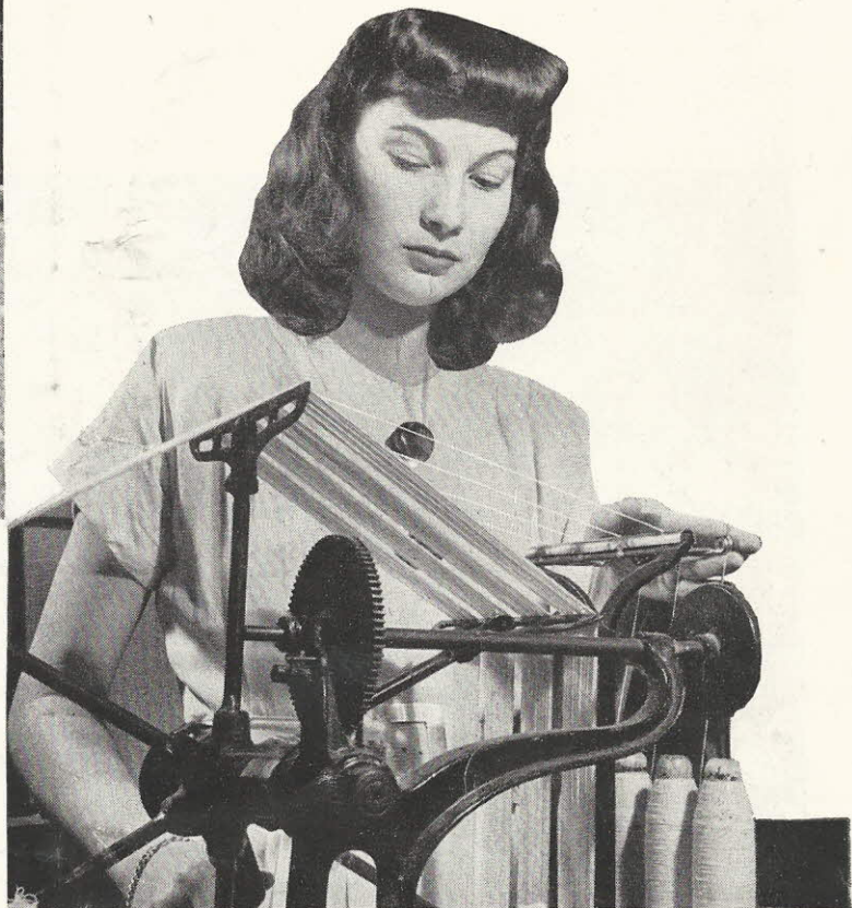
Winnsboro Mills is the first plant in our Textile division. Chief products of this plant are tire cord and fabric, Strex and Ustex. In the laboratory of the Winnsboro Mills Betty Mattox, above, reels single yarn into skeins, preparatory to testing for tensile strength on a yarn breaking machine.
