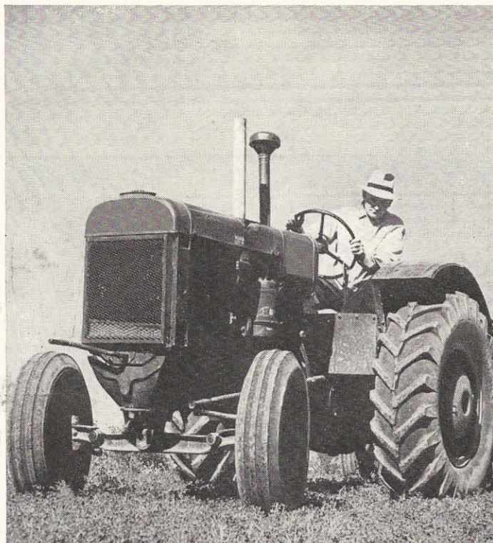
Different types of tires have different requirements. Especially designed for farm service is this strong, heavy tire with deep grooves to keep a tractor moving in soft soil. Truck tires have other requirements, such as stamina and resistance to heat.
