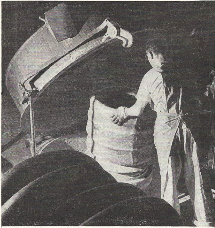
Shaping of the tire takes place in a huge vacuum box. The assembled tire, looking like a barrel without top or bottom, is put into the box by operator Al Boyer. Then the lid is closed and the air pressure forces the center of the tire outward to assume a doughnut shape.
