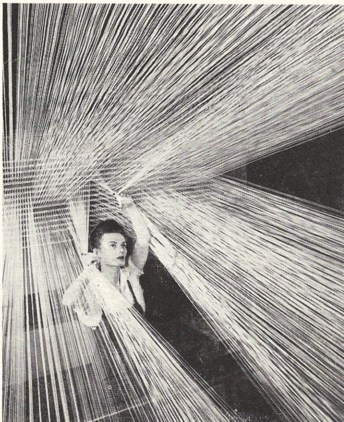
Textiles used in tire cord are assembled, as Clara Gerlach is doing, then dipped in latex, dried and given a further coating of rubber.
