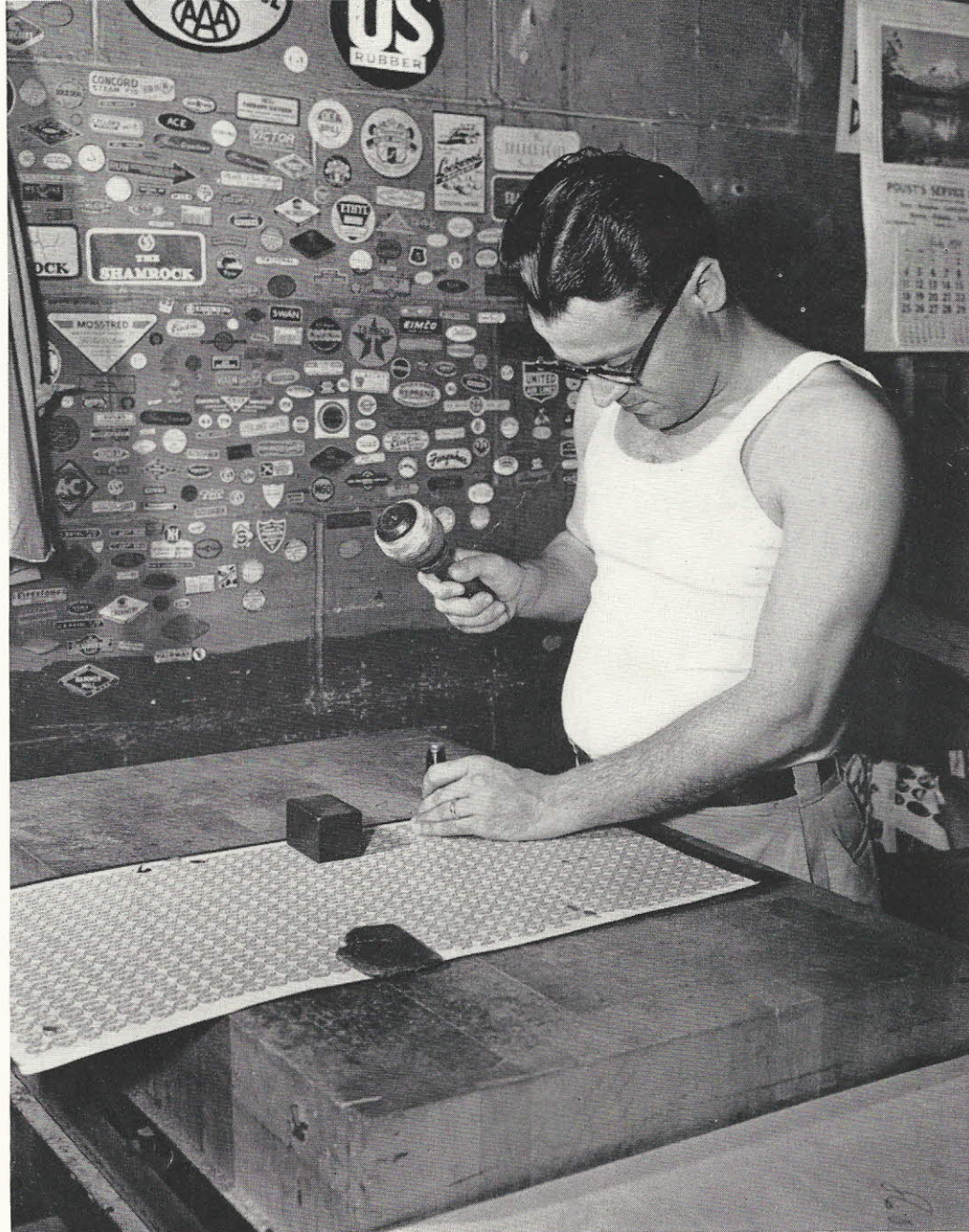
RUBBER LABELS —all sizes and shapes—are cut by hand by Dominic Angiolillo. Label samples on the wall are just a few of the thousands he has cut while at Naugatuck Chemical.
