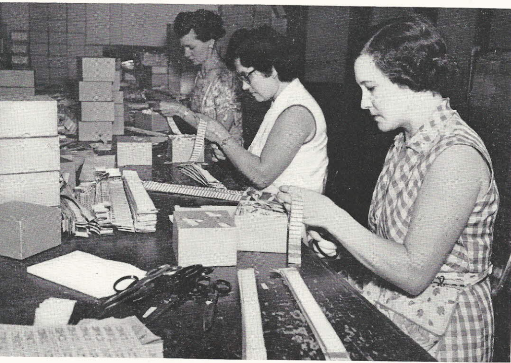
SQUARE or rectangular shaped labels are cut in strips and snipped with shears by (front to back) Mary Wailonis, Deolinda Pardal and Florence Kelsey.
