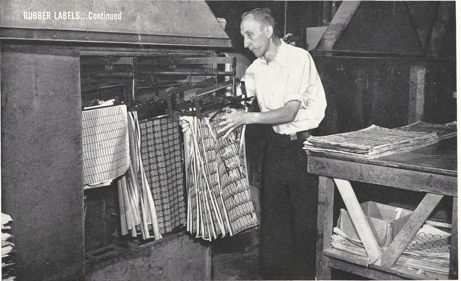
CURING BOXES partially cure labels for one hour at 190 degrees. Eitel Radwick removes a batch of cured labels ready for inspection.
